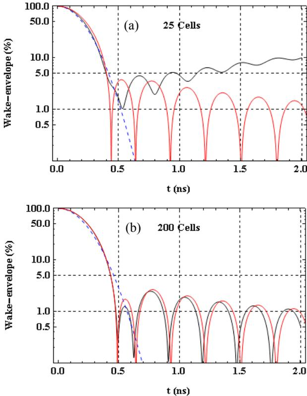
Figure 1 Uncoupled normalised and loss-less wake-field of 25 cell and 200 cell structures. The black, blue-dashed and red curves represent Eqs. 1 ( $\text{Im}$  replaced with  $\text{abs}$ ), 4 and 5 respectively. The Qs are assumed to be infinite.
