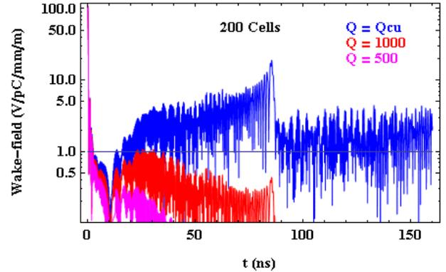
Figure 5: Wake-field of 200 cell structure with finite  $Q$ s.
