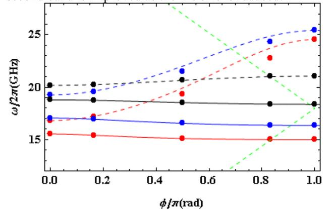
Figure 2: Dispersion curves of three cells. The points represent simulations and curves represent the circuit model. The red, blue and black represent geometries with  $a(\text{mm}) = 4.95, 3.95,$  and  $2.15$  respectively. The light line is shown dashed.
