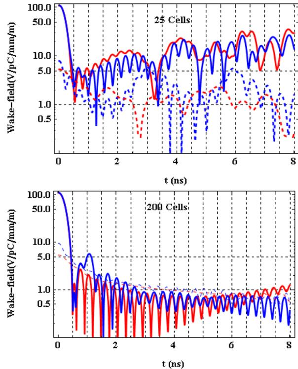
Figure 4: Wake-fields of 25, and 200 cell structures. The red and the blue curves represent the uncoupled and the coupled wake-fields respectively. The solid curves represent the wake-field of the first dipole band and dashed curves that of the second dipole band.
