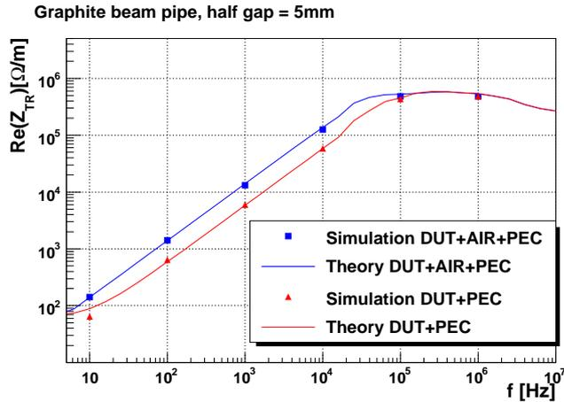
Figure 1: Real part of the transverse impedance as calculated by numerical simulations [4] and analytical models [1] for cylindrical graphite and copper beam pipes. PEC stands for Perfect Conductor
